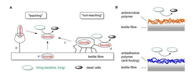
Figure 2. A: Different approaches to attach biocides to textiles using a chemical finishing process. B: Coating of textile fibres with antimicrobial or antiadhesive polymers.
