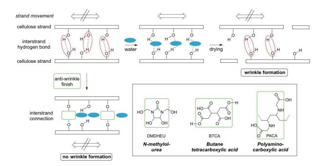
**Figure 1.** Mechanism of wrinkle formation (top), effect of anti-wrinkle finishes (bottom), and structure of chemicals that act as anti-wrinkle finishes (inset).
