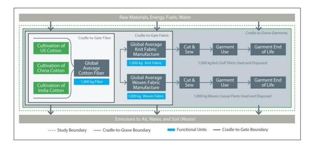
Figure 1. Vision 21 LCA system boundaries and functional units.
