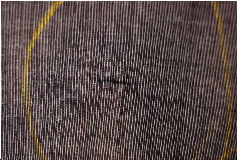
Figure 1. Spandex damages, yarns from tailored and washed trousers
