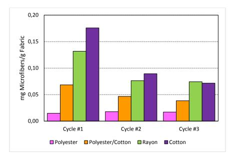
Figure 4. Microfibres Generated during Drying – Home Laundering.
