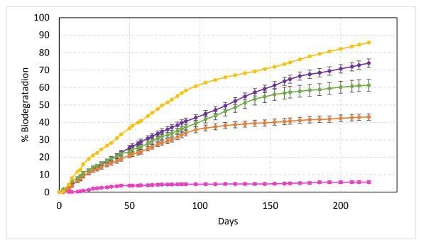
Figure 5. Biodegradation Results of Yarns in an aerobic aquatic environment (in decreasing extent of degradation: Microcrystalline cellulose, Cotton, Rayon, 50%/50% Polyester/Cotton, 100% Polyester).
