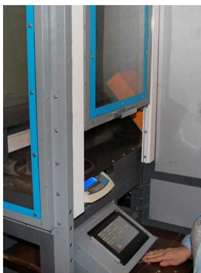
Fig.6 Instrument for determination of moisture (seed cotton, fiber, linter, seeds)
