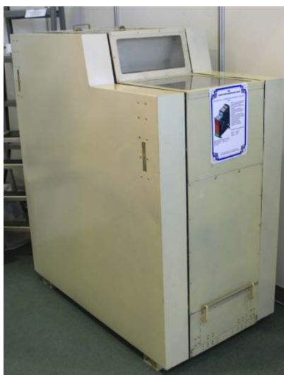
Fig.7 Automatic instrument for determination of seed cotton trash content
