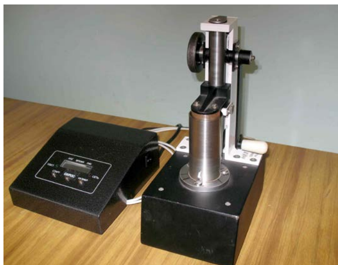
Fig.5 Instrument for determination of micronaire (acoustic method)
