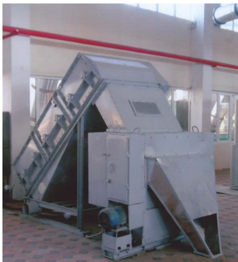
Fig.1 The new universal cleaner of cotton fiber materials
