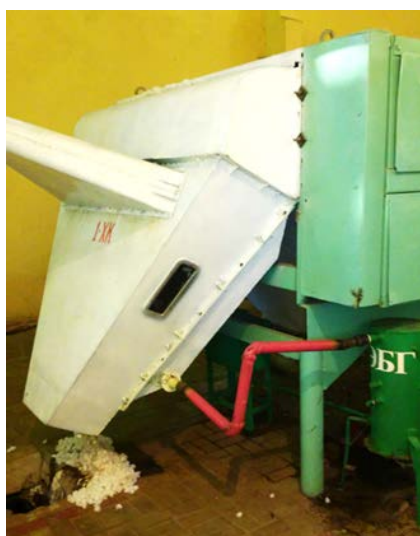
Fig.3 Humidifier of seed cotton on the unit "UHK" (1HK)
