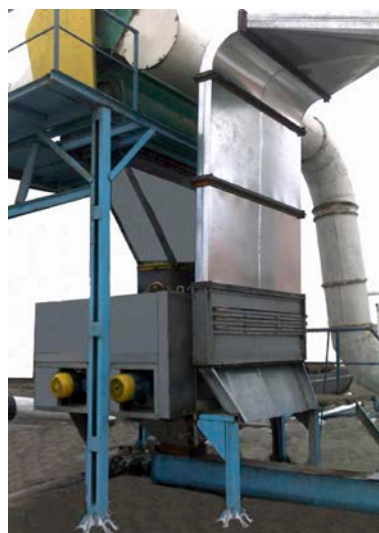
Fig.2 The new cleaner-trap of heavy impurities
