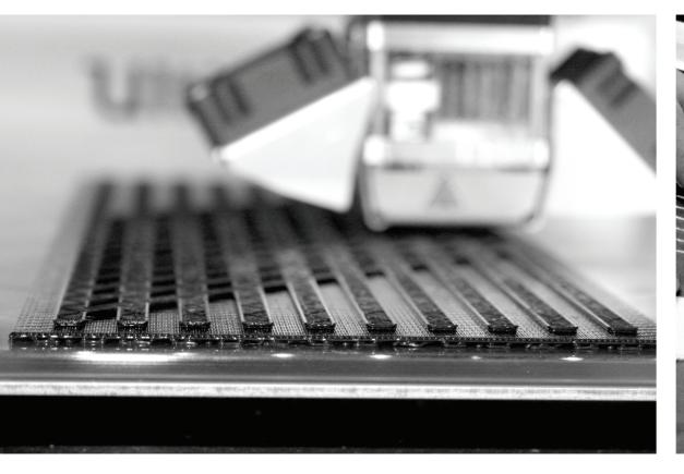
Melting process of fibres and PLA structure
