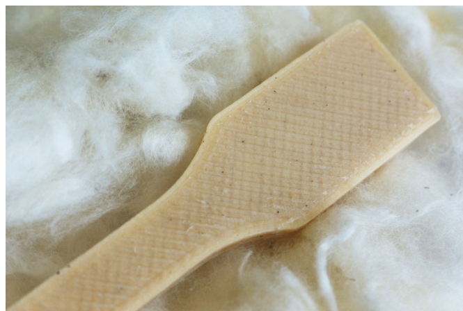
Figure 2: Tensile bar printed with a cotton fibre-reinforced thermoplastic wire.
