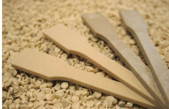
Figure 1: Pellets and injection moulded standard tensile testing bars made of cotton fibre-reinforced bio-based polymers.
