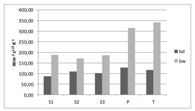
*Fig.* 8. *Thermal absorptivity of the investigated fabrics in dry and wet state: bd – in dry state, bw – in wet state*
