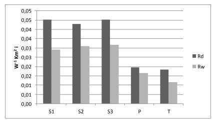
Fig. 6. Thermal resistance of the investigated fabrics in dry and wet state: Rd – in dry state, Rw – in wet state
