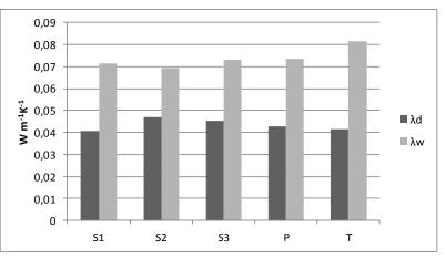
*Fig. 5. Thermal conductivity of the investigated fabrics in dry and wet state:*  $\lambda d$  – *in dry state,*  $\lambda w$  – *in wet state*
