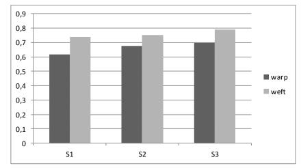
Fig. 10. Friction coefficients of the investigated seersucker woven fabrics
