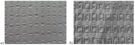
Fig. 4. The seersucker fabrics with seersucker effect in both directions: a) the sample S 2, b) the sample S 3
