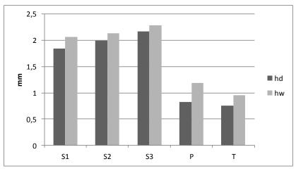
*Fig. 7. Thickness of the investigated fabrics in dry and wet state:* hd - in dry state, hw - in wet state
