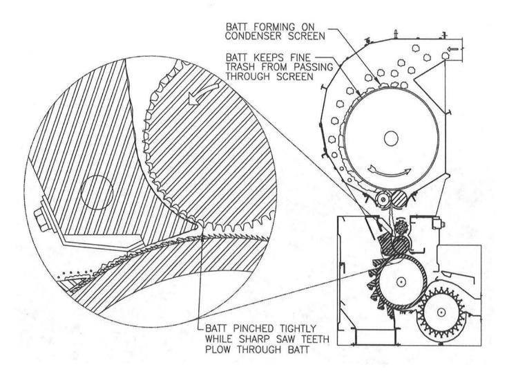
Figure 2. A typical conventional controlled-batt, saw-type lint cleaner (the Lummus Model 108 Lint Cleaner).
