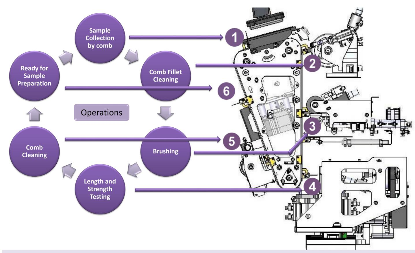
The Length and Strength Module of the HVT Genius 2 Fully Automatic Fibre Tester comes with a Rotosampler device capable of automatically preparing six combs in sequence and presenting the sample beards into the testing module.
