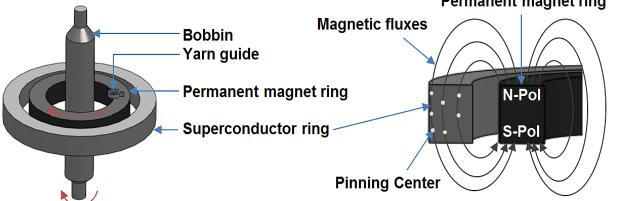
Concept 2: Topology and cross-sectional view, where magnetic fluxes are trapped in pinning center
