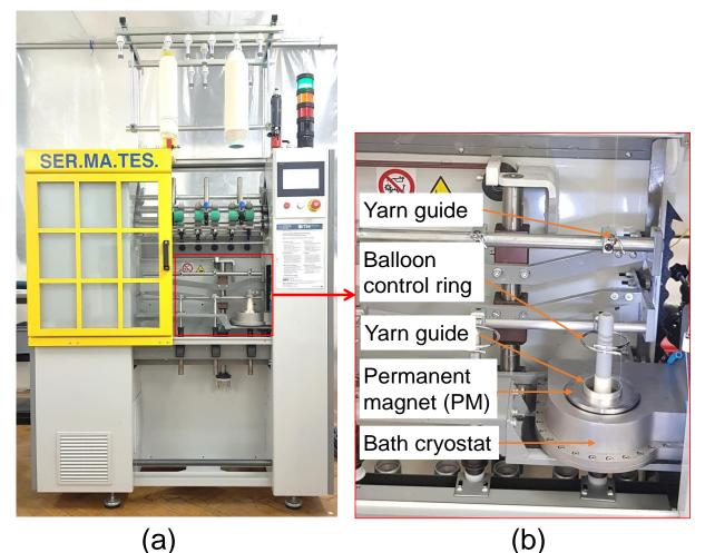
(a) Superconducting high performance ring spinning tester and(b) superconducting magnetic bearing (SMB) twisting system with bath cryostat
