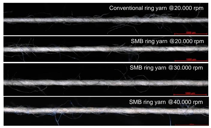
Comparison of yarn structure of conventional and SMB ring yarn from 100% cotton material for different angular spindle speeds (yarn count 20 tex)
