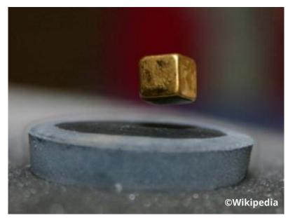
A magnet levitates above a high temperature superconductor cooled with liquid nitrogen (-196°C) PM: Permanent magnet HTSC: high temperature superconductor Cooling PM PM HTSC HTSC
