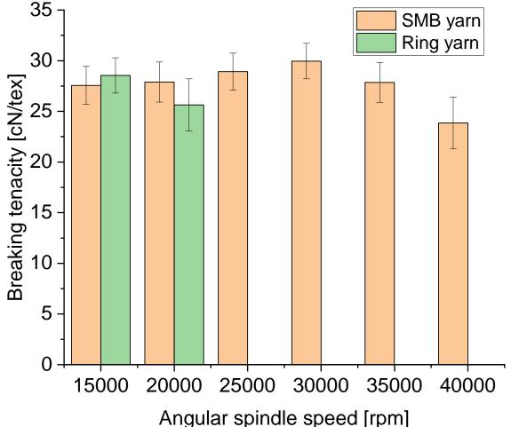
Comparison of yarn strength of conventional and SMB ring yarn from 100% cotton material for different angular spindle speeds (yarn count 20 tex)
