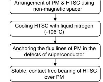
Functional principle of superconducting magnetic bearing (SMB)
