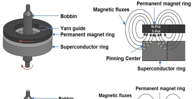
Concept 1: Topology and cross-sectional view, where magnetic fluxes are trapped in pinning center
