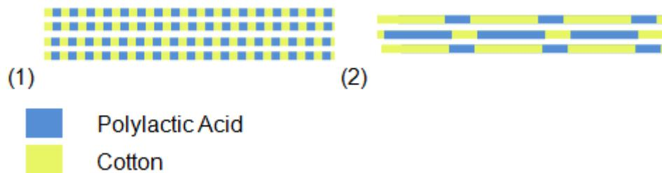
**Figure 4. Uniform (1) and Diverse (2) Laminate Structure**
