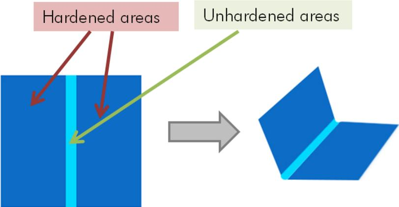
**Figure 2. Concept of THERMOLINK**
