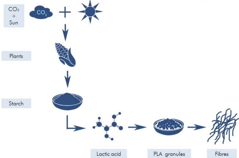
**Figure 1. Manufacturing Process of Polylactic Acid Fibres**
