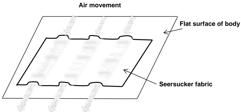
*Fig. 2. The scheme of air movement between the seersucker fabric and flat surface of human skin*
