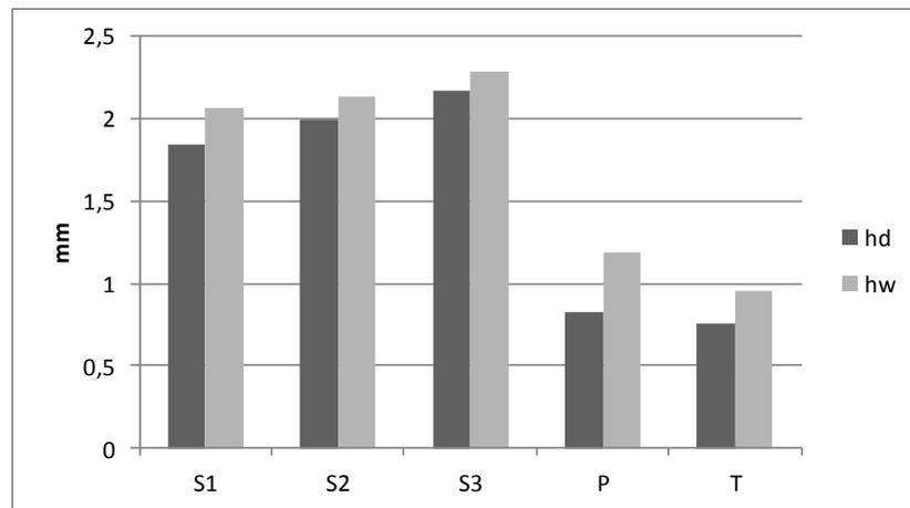
Fig. 7. Thickness of the investigated fabrics in dry and wet state:  $h_d$  – in dry state,  $h_w$  – in wet state
