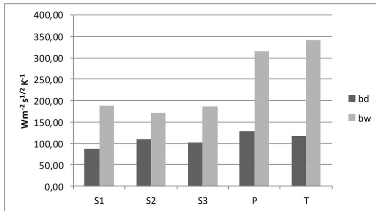
Fig. 8. Thermal absorptivity of the investigated fabrics in dry and wet state: *bd* – in dry state, *bw* – in wet state
