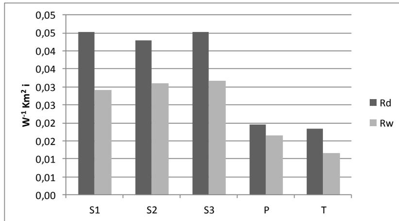
Fig. 6. Thermal resistance of the investigated fabrics in dry and wet state:  $R_d$  – in dry state,  $R_w$  – in wet state
