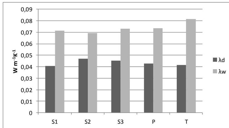
Fig. 5. Thermal conductivity of the investigated fabrics in dry and wet state:  $\lambda_d$  – in dry state,  $\lambda_w$  – in wet state
