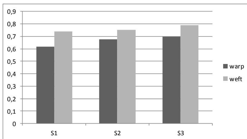
Fig. 10. Friction coefficients of the investigated seersucker woven fabrics
