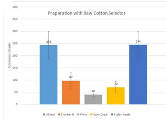
Fig. 5: Sample prepared with the RCS
