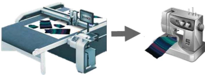
**Figure 5: Automated single-ply cutting and confection**
