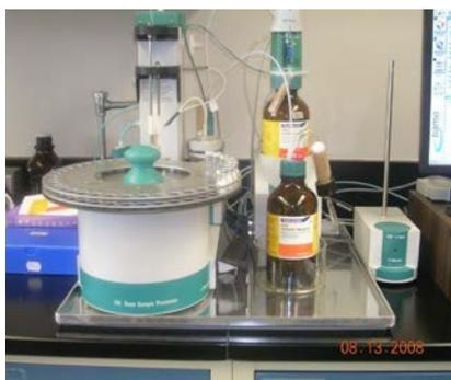
Figure 1. Set-up for the KFT fiber water content measurement.
