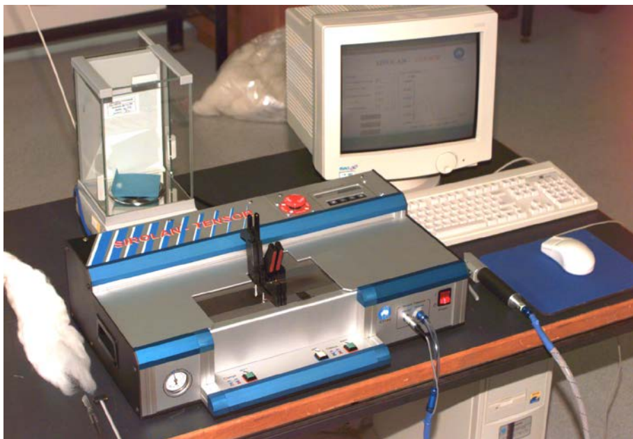
Figure 1(b) – CSIRO Sirolan-Tensor instrument
