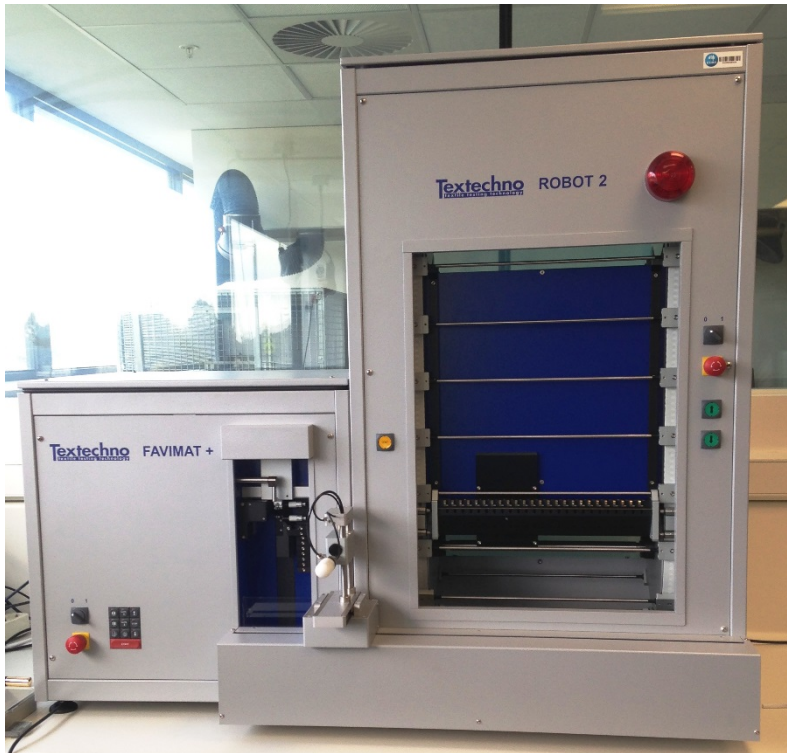
Figure 1(a) – Textechno Favimat instrument
