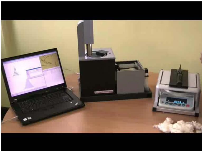
**Figure 1.** Cottonscope (computer, water base unit, knife blade cutter).
