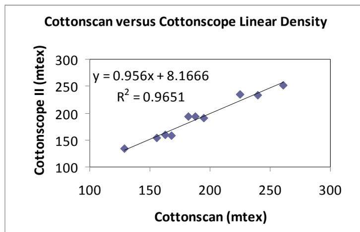
**Figure 8.** Average fibre fineness (linear density) values measured on the Cottonscope plotted against the published values (Abbott et al, 2011).
