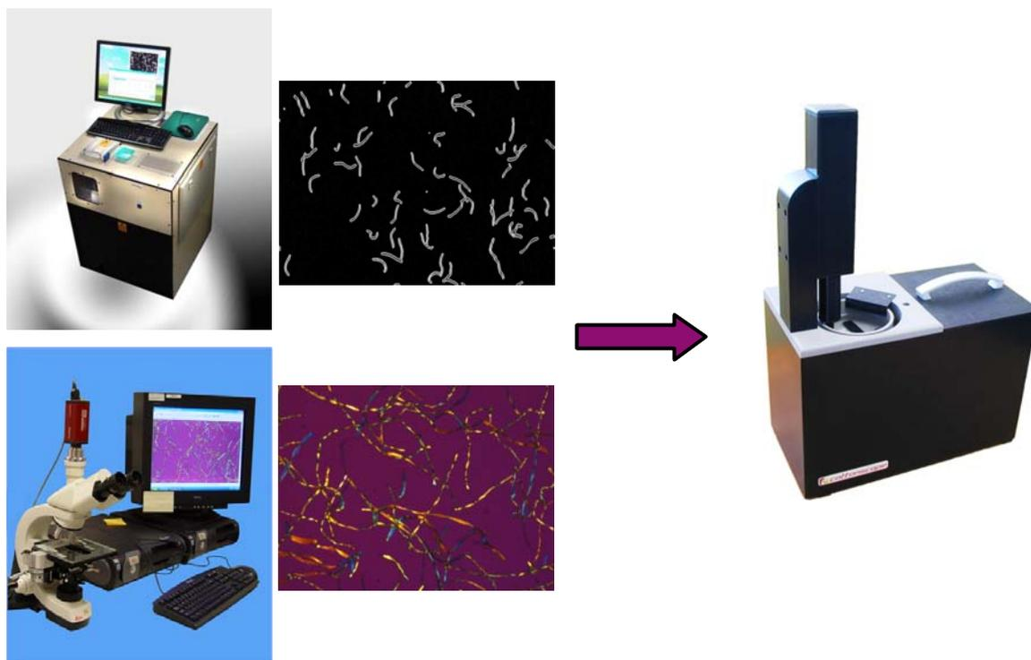
**Figure 4.** Creation of Cottonscope through the innovative merging of the Cottonscan™ and Siromat™ technologies.
