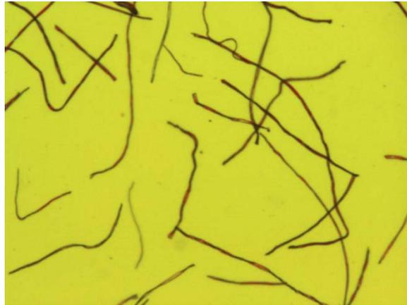
**Figure 6.** Typical Cottonscope image of cotton snippets.
