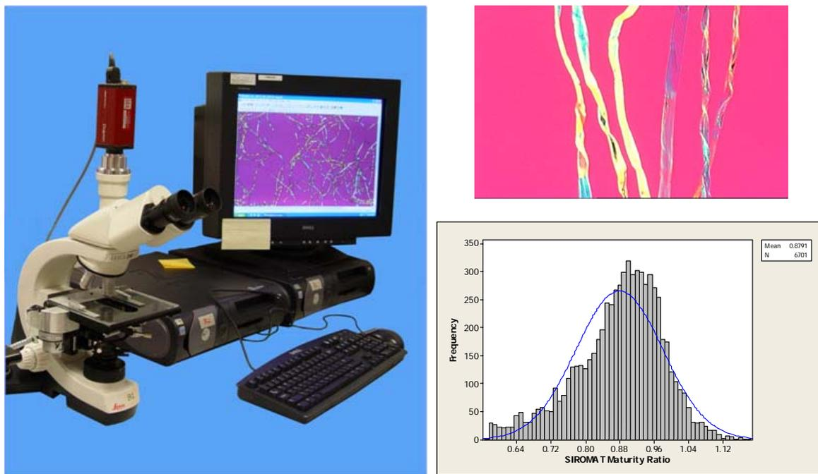
**Figure 2.** The Siromat™ Technology and Instrument. The polarising microscope, colour digital camera and computer system are shown on the left. The top right frame is an image illustrating the difference between mature and immature fibres (mature fibres on the left and immature fibres on the right). The bottom right frame depicts the histogram output of maturity values within a sample available from the technology.
