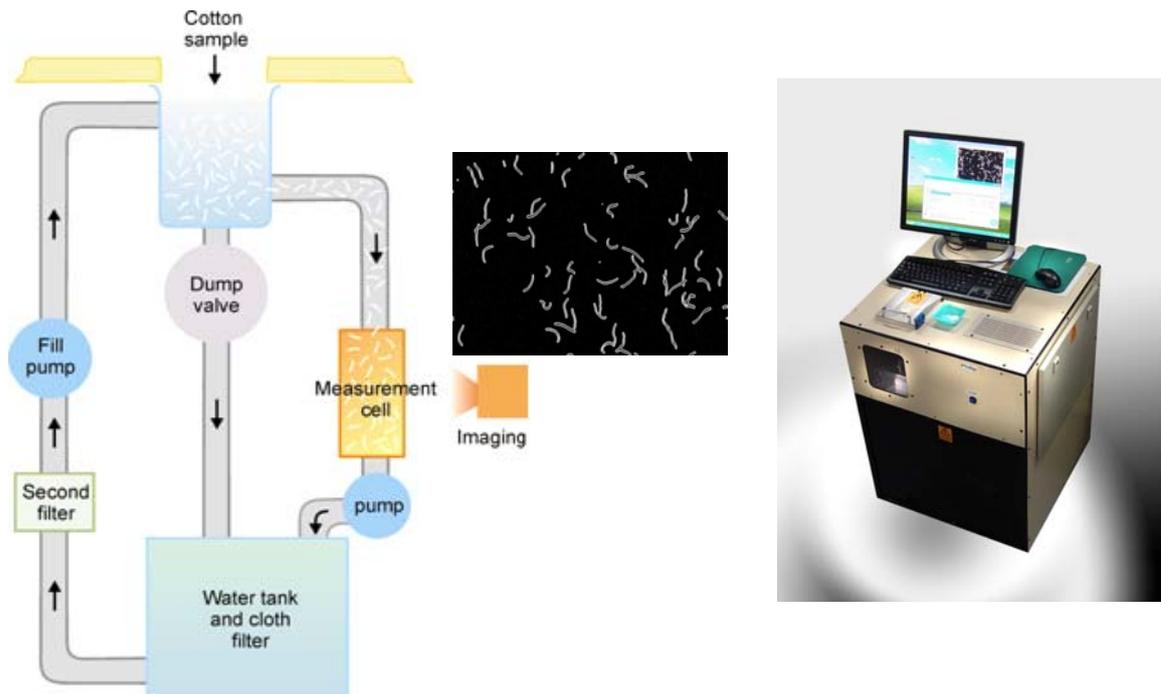
**Figure 3.** The Cottonscan™ Technology and Instrument. A schematic of the operation of the instrument is shown on the left. The centre frame is a typical black and white image of the suspended snippets as they pass the measurement cell. The frame on the right depicts the instrument.
