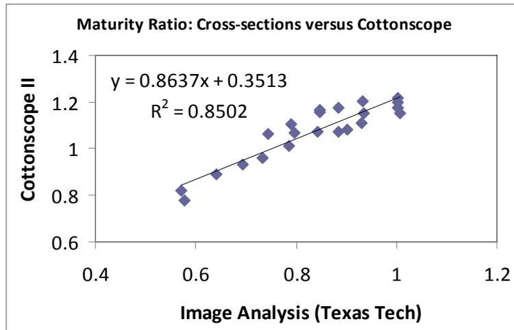
**Figure 7.** Average fibre maturity measured on the Cottonscope plotted against the published values (Hequet et al, 2006).
