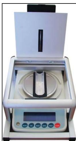
**Figure 5.** The custom designed 0.7 mm guillotine mounted above the snippet weighing balance. The image shows the underside of guillotine slot and collection trough on the balance.
