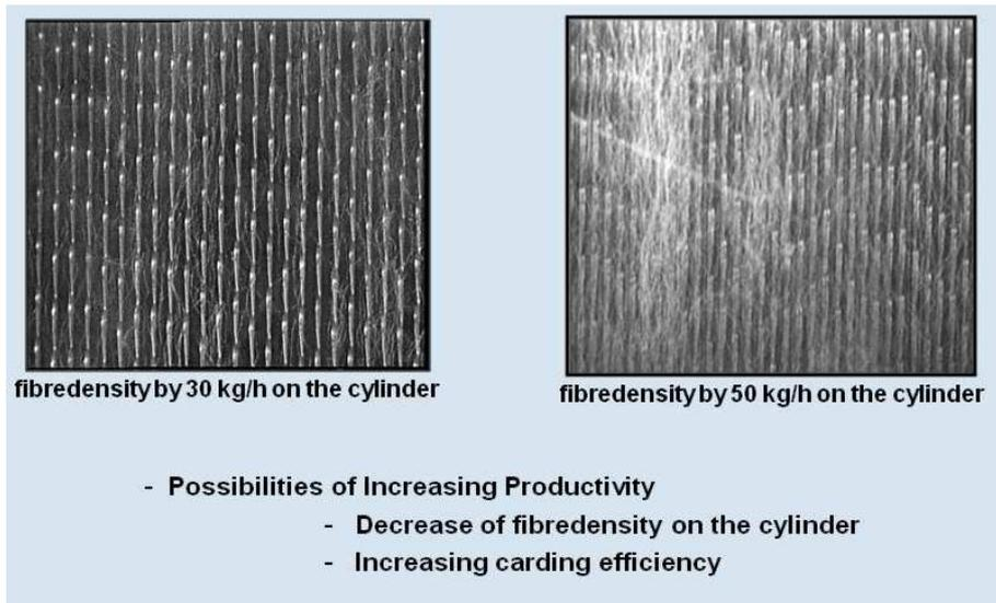
**Fig.: 1 Fibre density on the cylinder**
