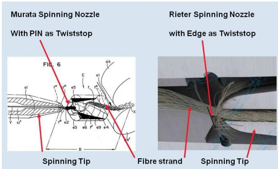
**Abb.: 3 Differences in the nozzle design**
