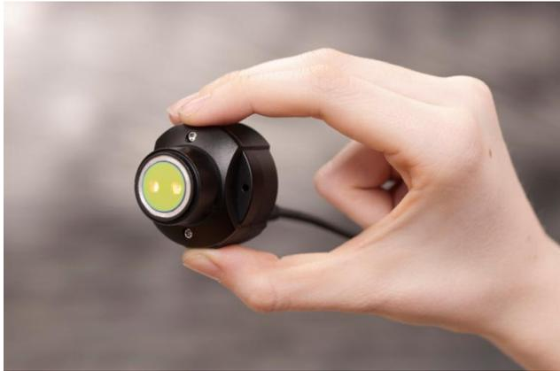
**Figure 8.** JDSU MicroNIR™ portable NIR unit.
