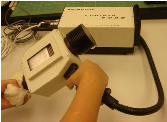
**Figure 5.** Brimrose Luminar™ 5030 portable NIR unit.
